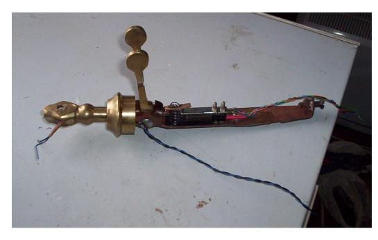
The dial didn't seem very good. This was an ITI (Indian Telephone Industries) version of an ATE one.<sup>\*</sup> My luck continued as I'd got a broken ATE one and the ITI one provided the bit I needed to fix it.
