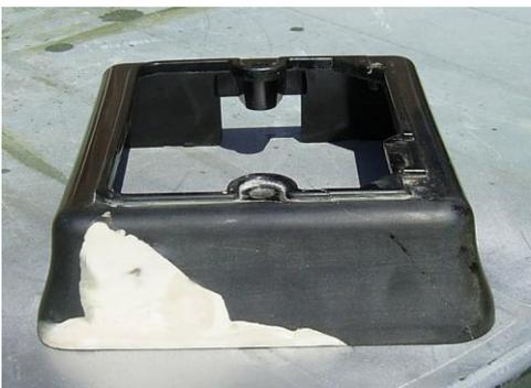
I superglued the broken part back which held it in place well enough to get some fibreglass behind it. I also used fibreglass to bridge the gap and then brought it up to level with Isopon P38 car filler. I could have attempted to stain this black but I know from experience that matching the colour is less than half the battle as fillers and substrates rarely polish to the same degree of shine. I therefore simply spray-painted the repaired side.
