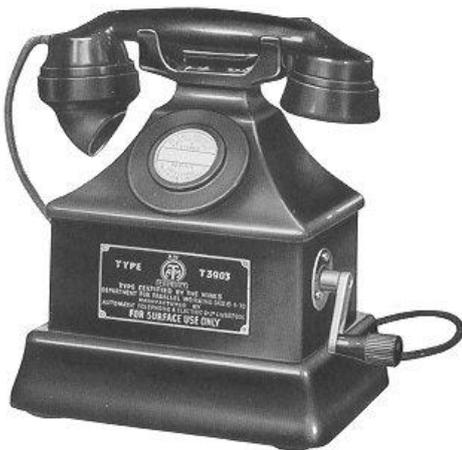
There was nothing I could do about the missing Certification Plate and as the magneto unit was just a great heavy lump of uselessness (sticking 90VAC up a telephone exchange or ATA isn't to be recommended!) I decided to remove it and configure it as a GPO 232.
