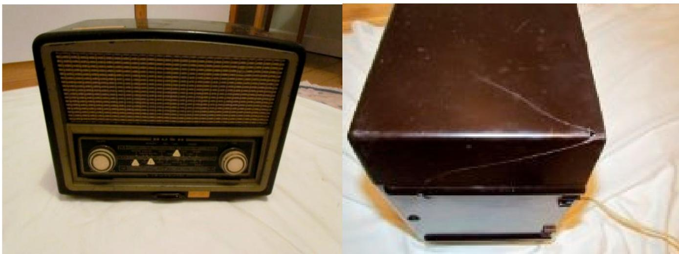
The case was cracked along one side and the bottom. The side stuck with epoxy but the bottom repair kept breaking again so I reverted to my old technique of sticking the edges with super-glue and then reinforcing the inside with glue-gun glue, like applying a weld. With this being at the bottom it won't get hot enough to melt.
